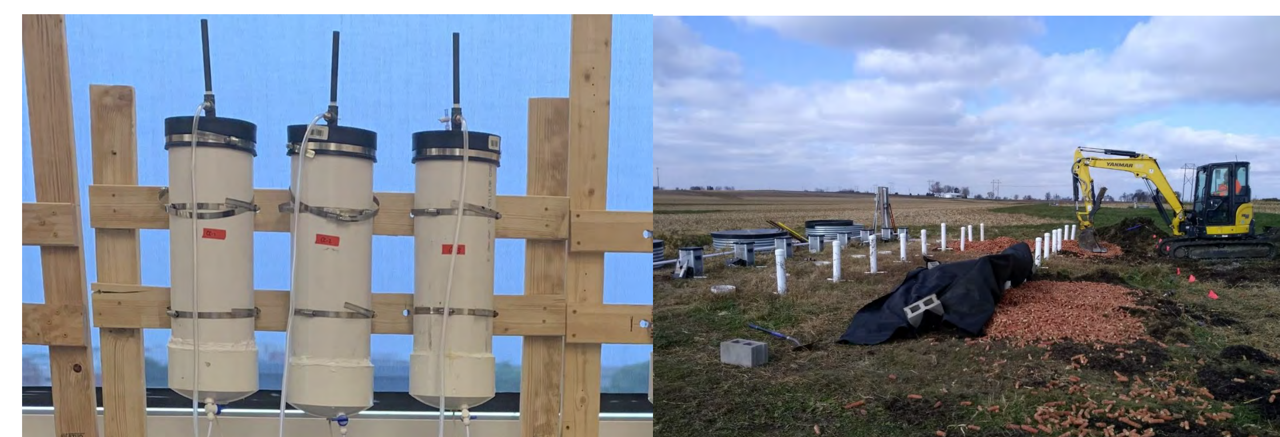
Lab up flow columns packed with woodchips
